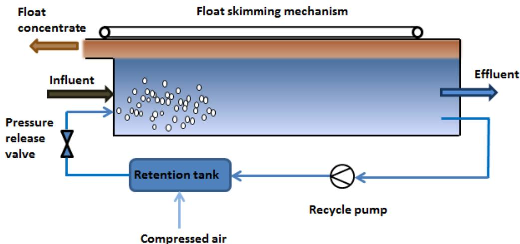
**Figure 9: Schematic description of dissolved air flotation (DAF) with effluent recycling, adapted graphic<sup>14</sup>**
