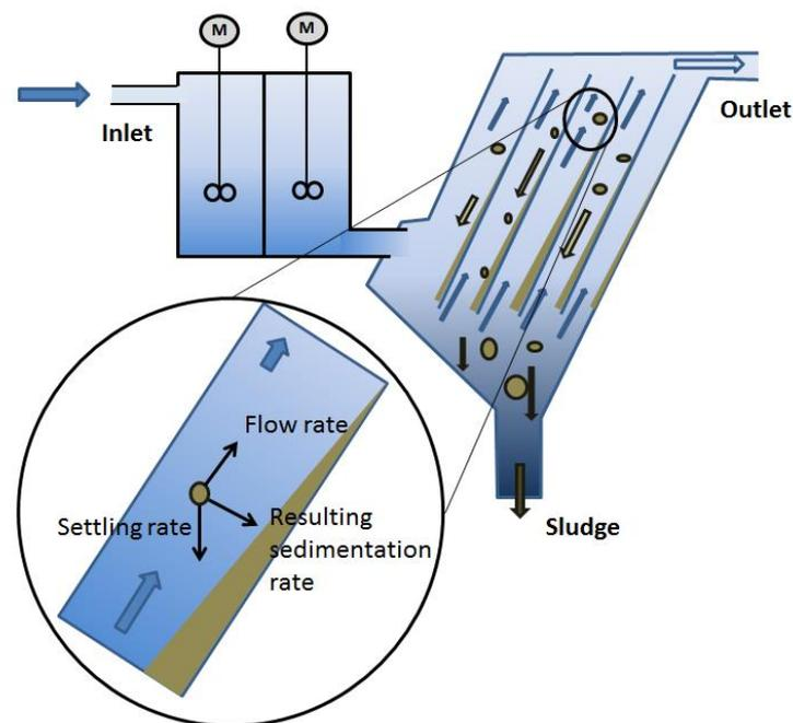
**Figure 5: Schematic description of a cross-current lamella settler including chemical dosing, adapted graphic<sup>6</sup>**
