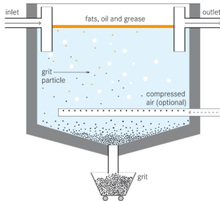
**Figure 2: Schematic description of a grit chamber<sup>2</sup> (other tank designs possible).**
