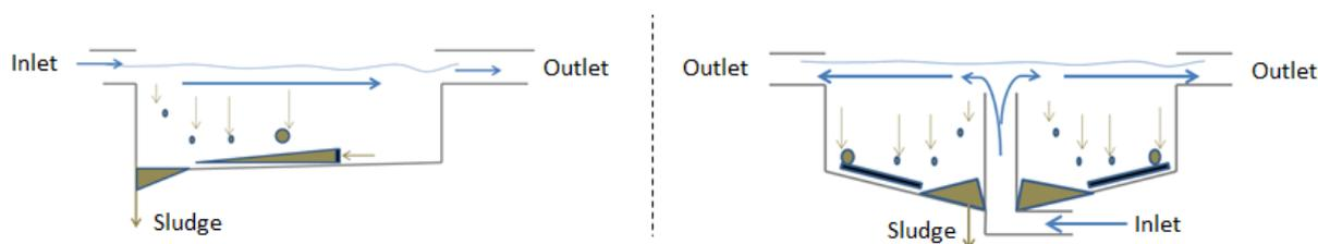
**Figure 3: Schematic description of rectangular and circular PSTs.**
