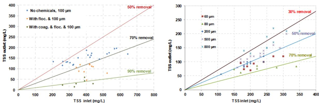
**Figure 7: right: TSS removal in the filter depending on the pore size of the filter material; left: TSS removal at different chemical pre-treatment options (WWTP Lynetten, Denmark, data collected in the “Avera Project”)**
