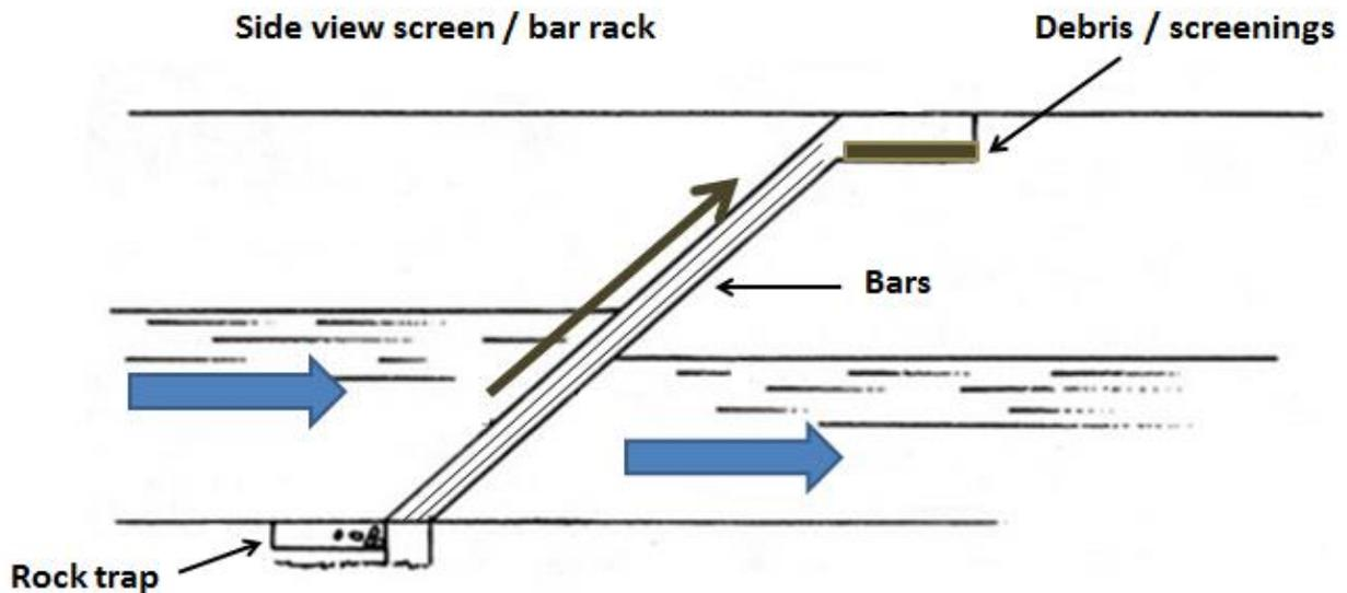
Figure 1: Scheme showing the side view of a screen / bar rack (adapted graphic)<sup>1</sup>
