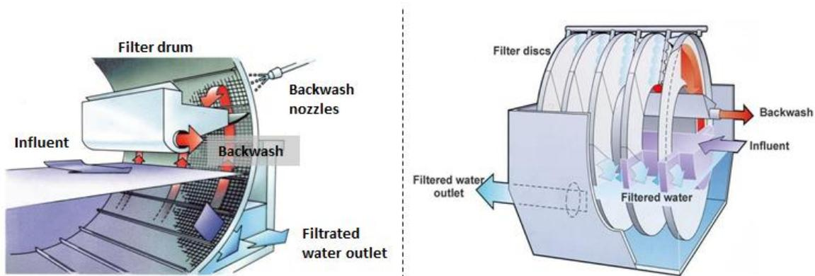
**Figure 6: Schematic illustration of a drum- (left) and a discfilter (right)<sup>9</sup>**
