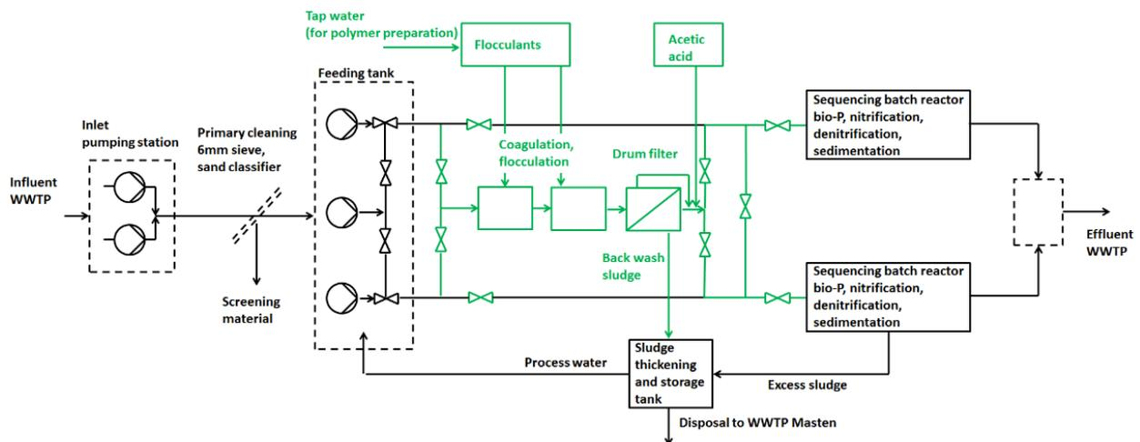
Figure 6: Process flow diagram of the WWTP Westewitz with advanced primary treatment
