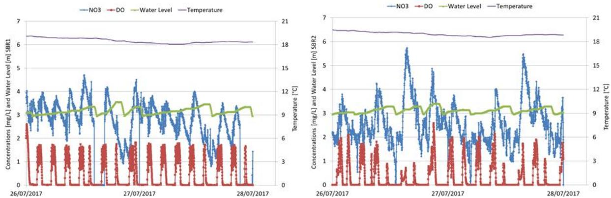
Figure 20: Operational data for SBR 1 and 2 at 42% COD load reduction
