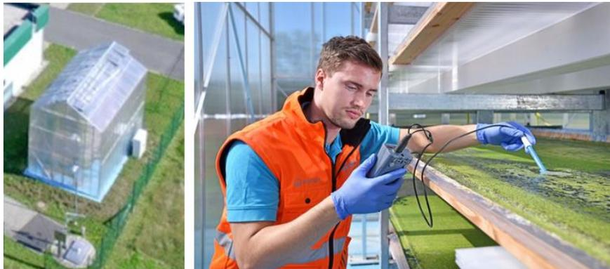
**Figure 4: left: Aerial image of the full scale duckweed pilot plant on Case study 1 (WWTP Westwitz, Germany); right: Measurement of the pH value in the duckweed trays within the plant**
