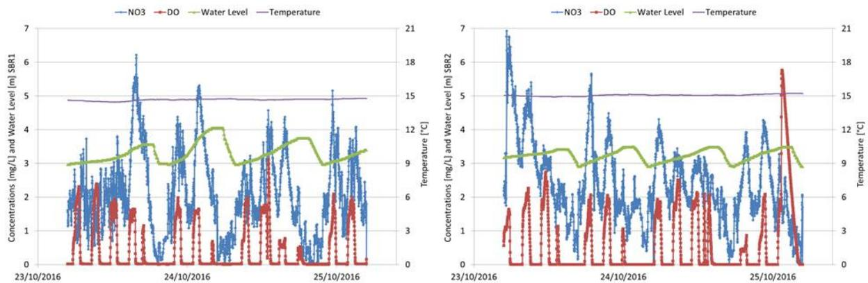
**Figure 18: Operational Data for reference Phase in SBR 1 and 2**
