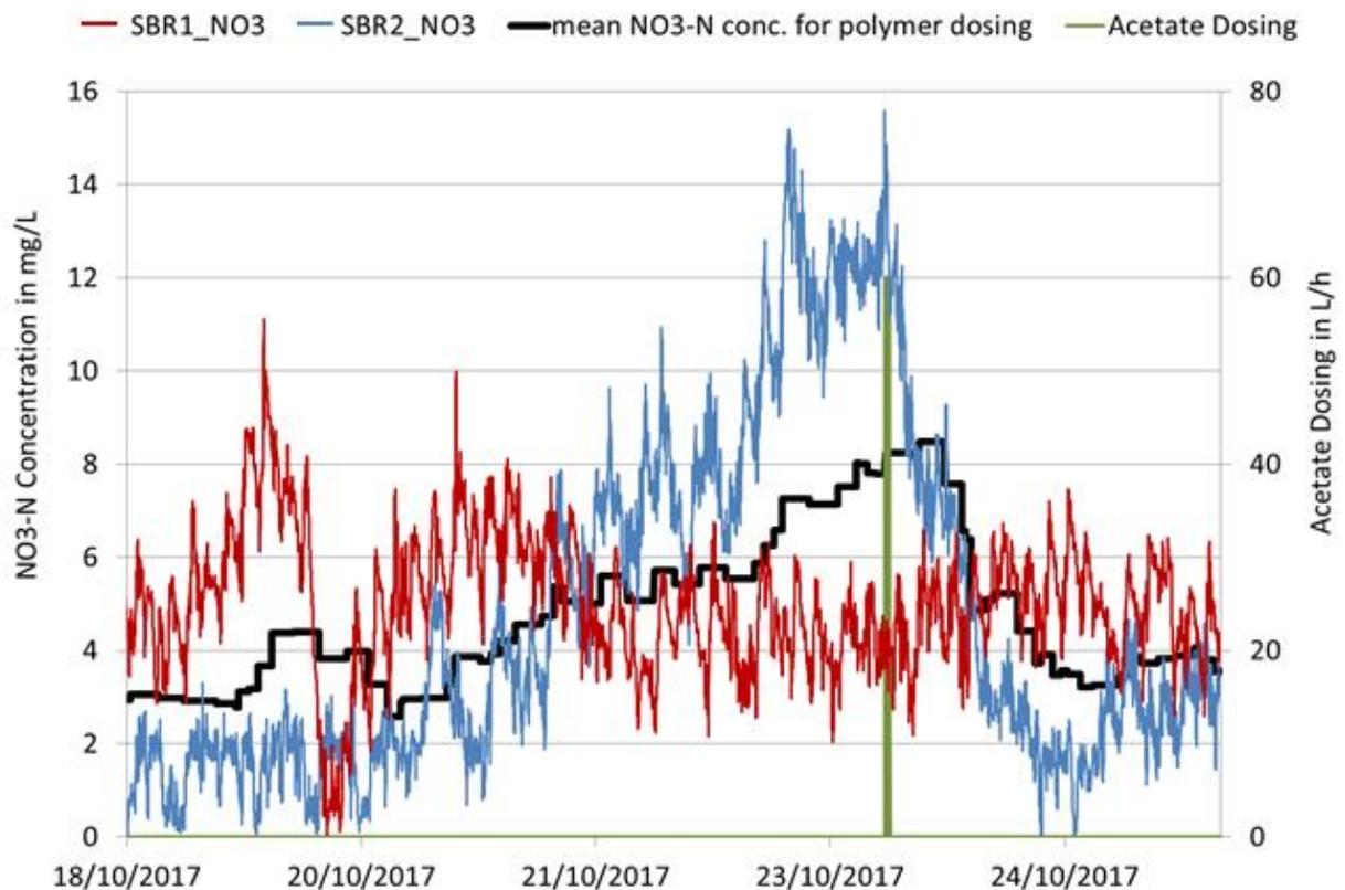
**Figure 23: Operational data during and after ammonium accumulation, for SBR1 and 2 mean nitrate concentration as a moving average of five values shown, monitored values of mean nitrate concentrations in both SBRs relevant for nitrate based polymer dosing indicated by the black line**
