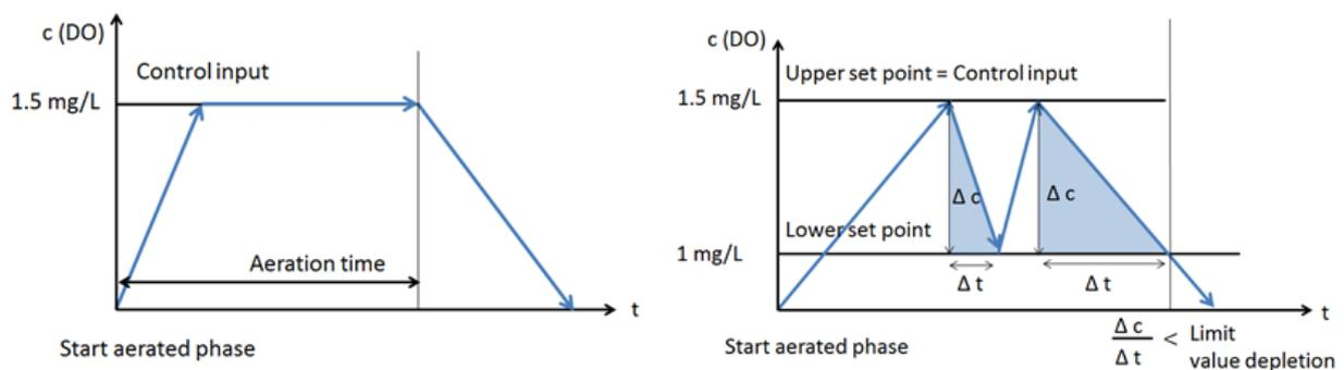
Figure 11: left: Scheme explaining the functionality of the time based oxygen control; right: Scheme explaining the functionality of the depletion based oxygen control
