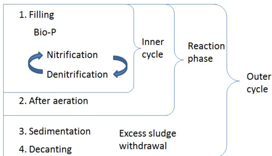
**Figure 10: Classification of the different phases within a cycle of SBR operation**
