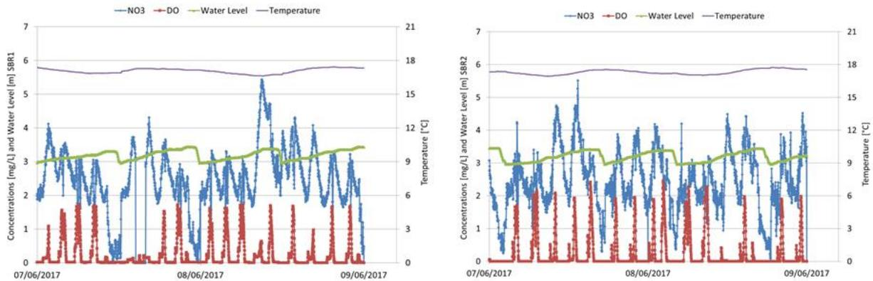
Figure 19: Operational data for SBR 1 and 2 at 30% COD load reduction
