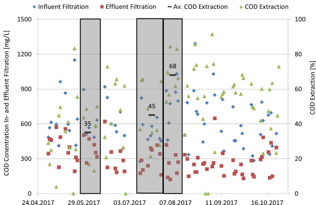
**Figure 17: COD concentrations of in- and effluent to filtration and time periods chosen for evaluation of denitrification rates (grey) with average COD extraction**
