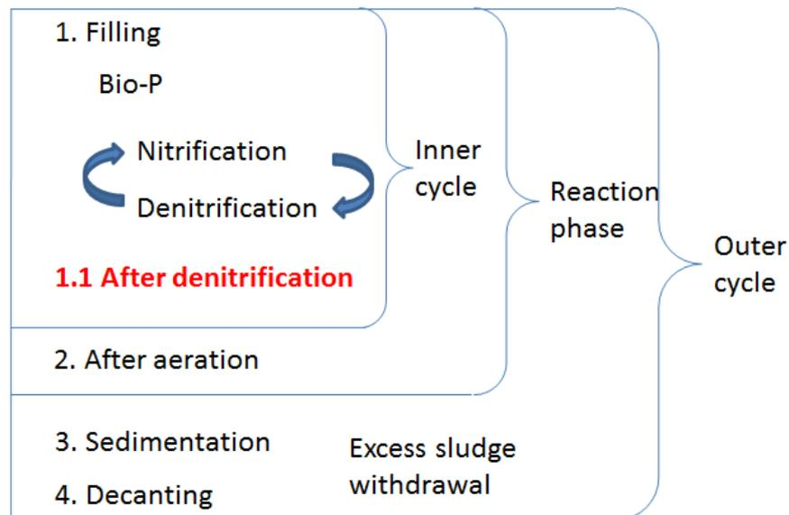
**Figure 15: Classification of the different phases within a cycle of SBR operation with added “After denitrification” phase (red)**
