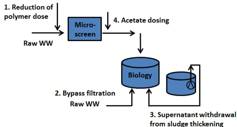
Figure 1: Schematic description of special mechanisms for advanced nitrogen control
