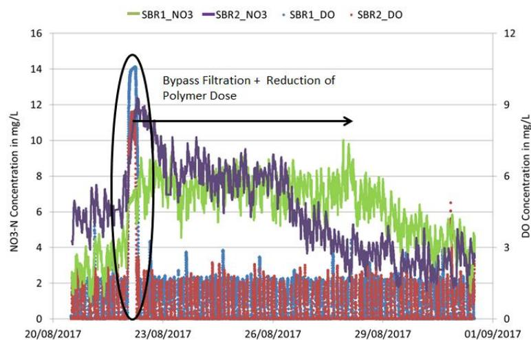
**Figure 22: Operational data SBR 1 and 2 during and after permanent aeration. Time of permanent aeration encircled in black**
