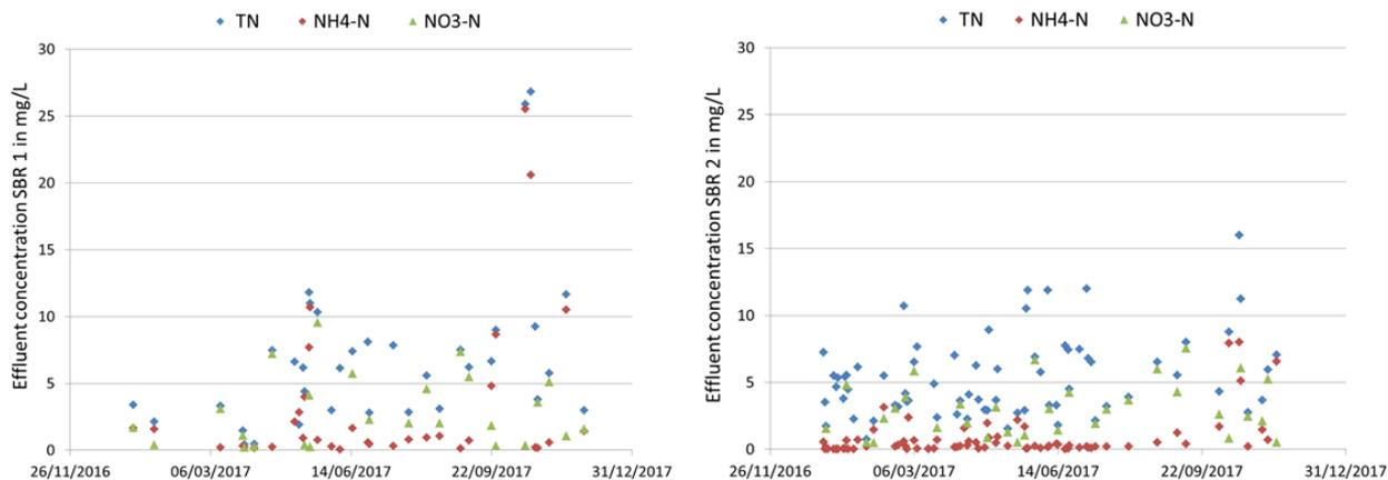
Figure 16: Effluent quality SBR 1(left) and SBR 2 (right) for different nitrogen fractions from Jan 2017 - Nov 2017
