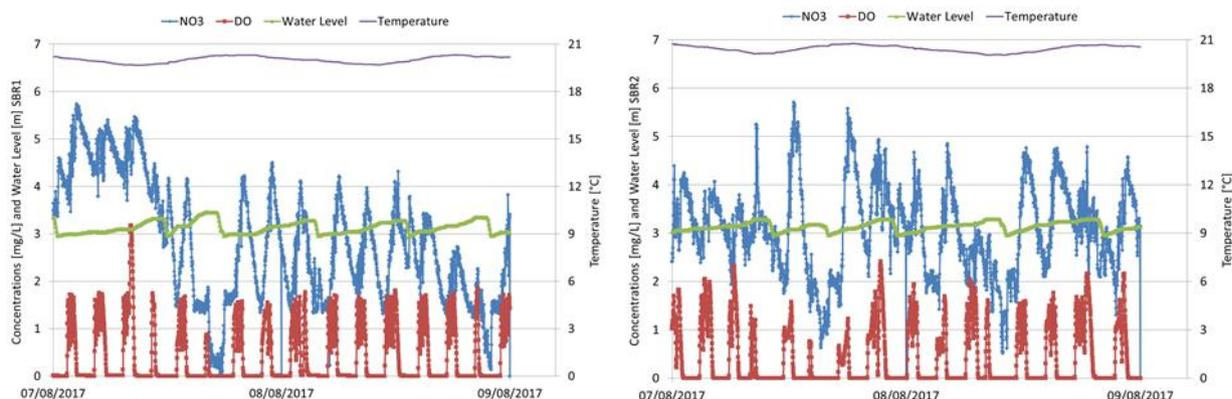
Figure 21: Operational data for SBR 1 and 2 at 58% COD load reduction
