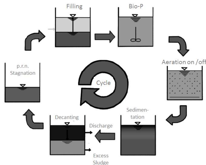
**Figure 9: Scheme of the phases within a cycle of SBR operation (modified graphic from DWA-M 210 (2009))**
