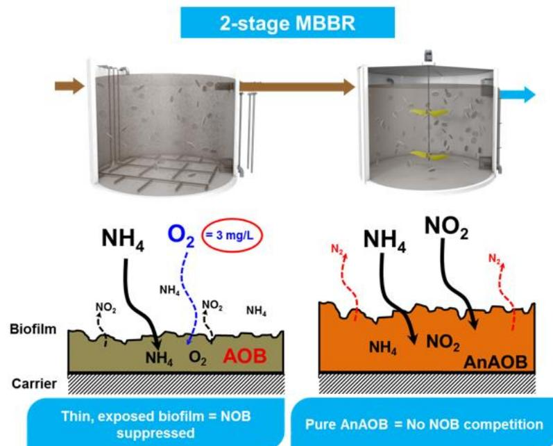
**Figure 3: Schematic description of the two stages of the anammox process and the corresponding biofilm characteristics. Left: First step: Nitritation under aerobic conditions (NOB: Nitrite oxidizing bacteria; AOB: Ammonium oxidizing bacteria); right: Second step: anammox reaction under anoxic conditions**
