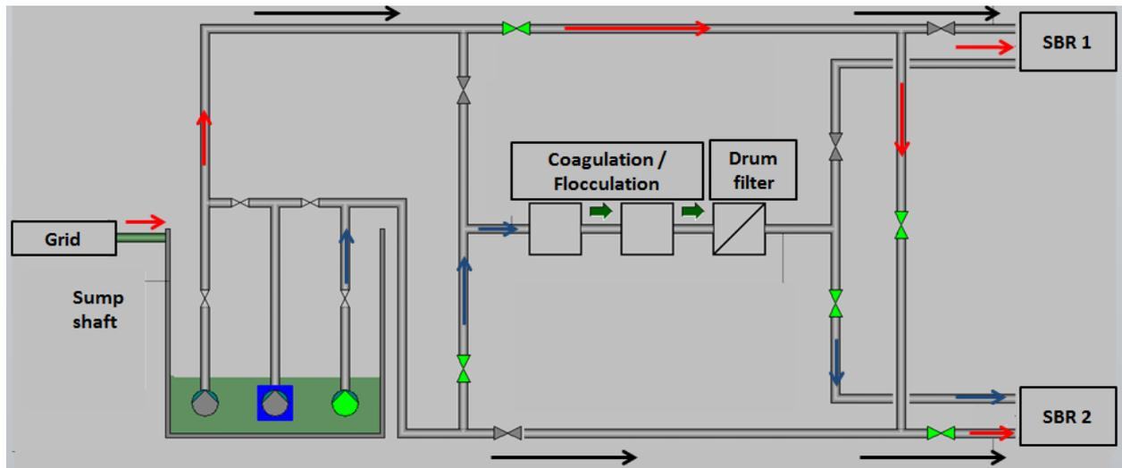
Figure 12: Screenshot from the PCS: Grid and sump shaft with drum filter and SBRs. Blue arrows: Pumping to the drum filter and SBR fed with filtrated water; red arrows: direct feeding of the SBRs with 2nd pump parallel to the drum filter operation; black arrows: direct feeding of both SBRs, no filtration
