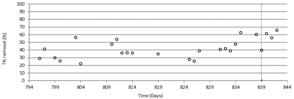
**Figure 21: Total nitrogen removal (%) in the one-stage IFAS MBBR during mainstream operation: The dashed line represents the switch from HRAS effluent to effluent from the Hydrotech drumfilter.**
