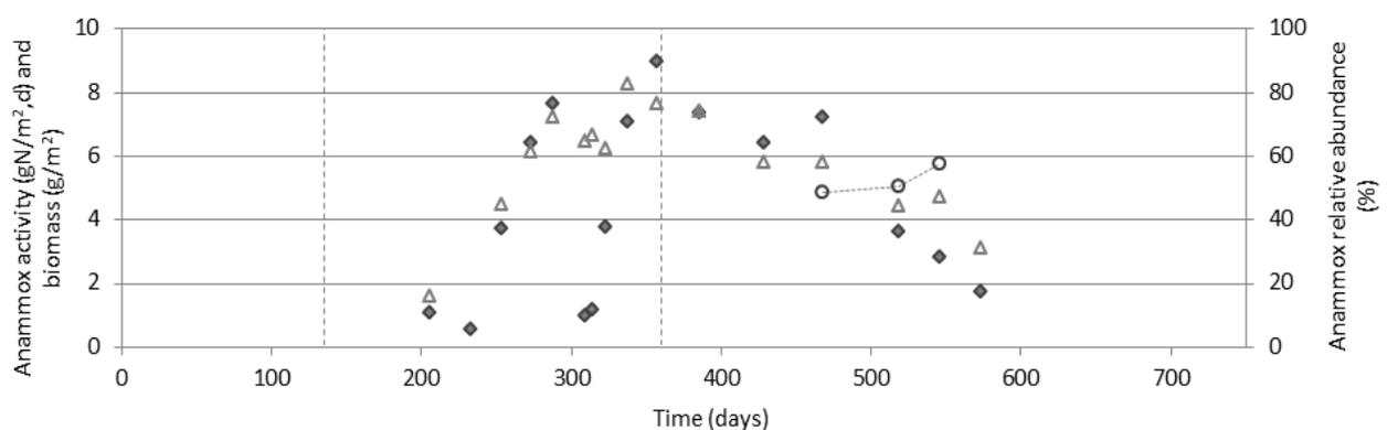
**Figure 15: Observed anammox activity in batch trials (diamonds), measured biomass (triangles) and relative abundance of anammox bacteria from DNA sequencing (circles) in carriers from the AMX-stage over time. Dashed vertical lines represents start-up of reactor (day 135) and connection with N-stage (day 360)**
