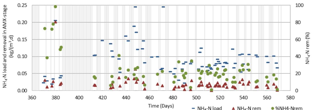
**Figure 10: Load, removal rate and efficiency in the AMX-stage during continuous operation on mainstream water (vertical grey lines represent days with reject operation when the AMX-stage was by-passed except during day 390-410 were the AMX-stage was fed reject water).**
