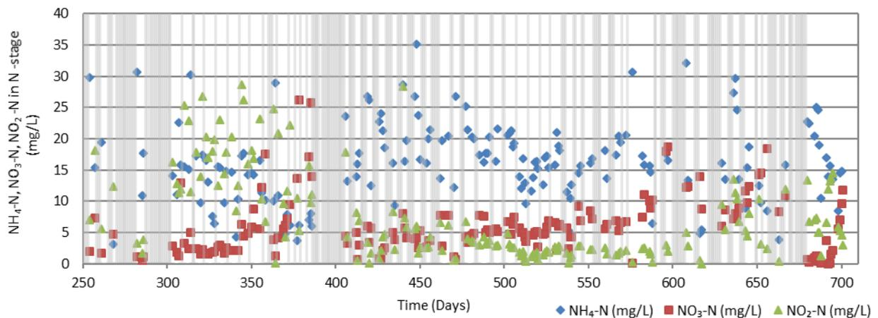
**Figure 9: Reactor concentrations in the N-stage during continuous operation on mainstream water (vertical grey lines represent days with reject feed). The y-axis is limited to 40 mg/L hence, the concentrations during reject water feeding are not shown in the figure.**
