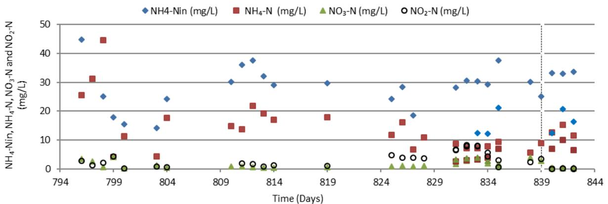
**Figure 20: Influent and effluent concentrations in the one-stage IFAS MBBR during mainstream operation. The dashed line represents the switch from HRAS effluent to effluent from the Hydrotech drumfilter.**
