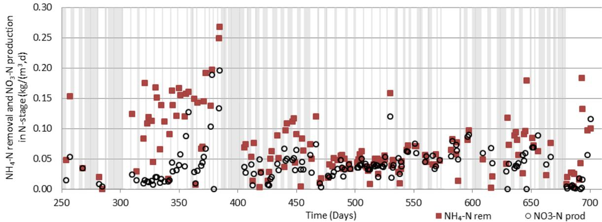
**Figure 8: Removal rates and production rates in the N-stage during continuous operation on mainstream water (vertical grey lines represent days with reject feed).**
