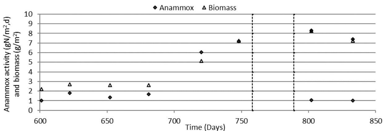
**Figure 24: Observed anammox activity in batch trials (diamonds) and measured biomass (triangles) in carriers from the one-stage IFAS reactor over time. Dashed vertical lines represents connection to the settler (day 758) and start of mainstream operation (day 789)**
