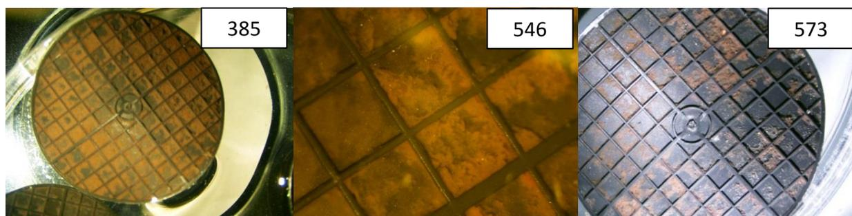
**Figure 17:** The biofilm on Anox K™ Z-400 carriers from the anammox reactor seen from above using a stereomicroscope on different operational days during mainstream operation.
