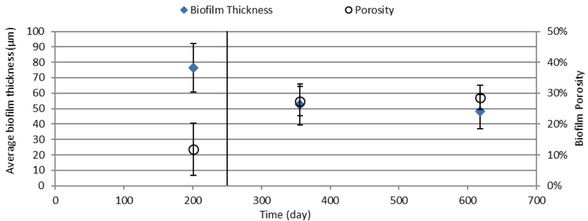
**Figure 14: The average biofilm thickness and porosity of Anox K™ Z-200 carriers from the N-reactor sampled at three different operational days, as analysed using OCT imaging. The black line represents the day when mainstream operation was initiated.**
