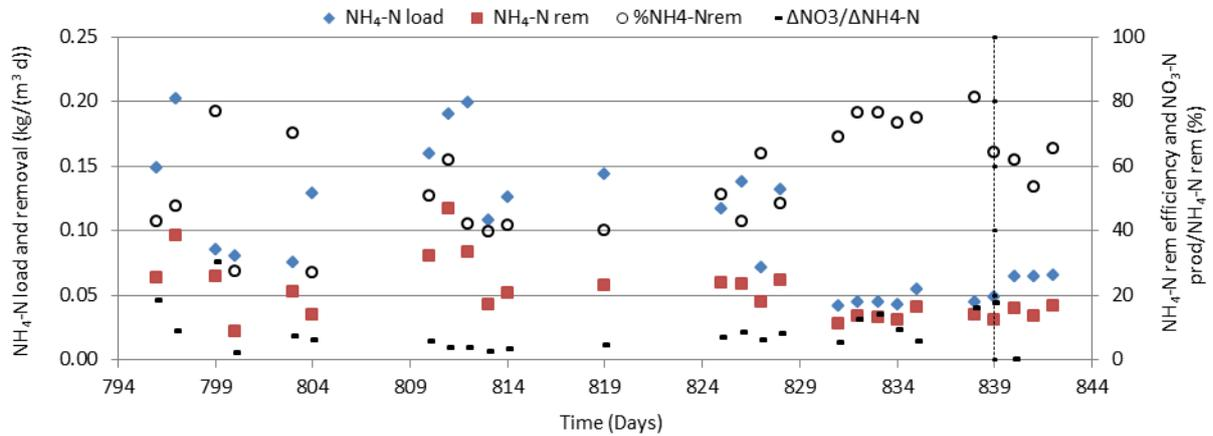
**Figure 19: Ammonia load, ammonia removal and produced nitrate over reduced ammonia during mainstream feed. The dashed line on day 839 represents the day when the IFAS was connected to the Hydrotech drumfilter.**
