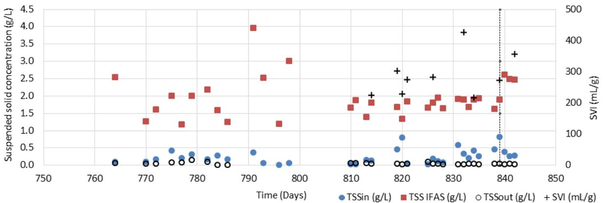
**Figure 22: Concentration of suspended solids in the influent, IFAS reactor and effluent (g/L) and SVI (mL/g) sampled during mainstream operation. The dashed line represents the day when the feed was changed to effluent from the Hydrotech drumfilter.**
