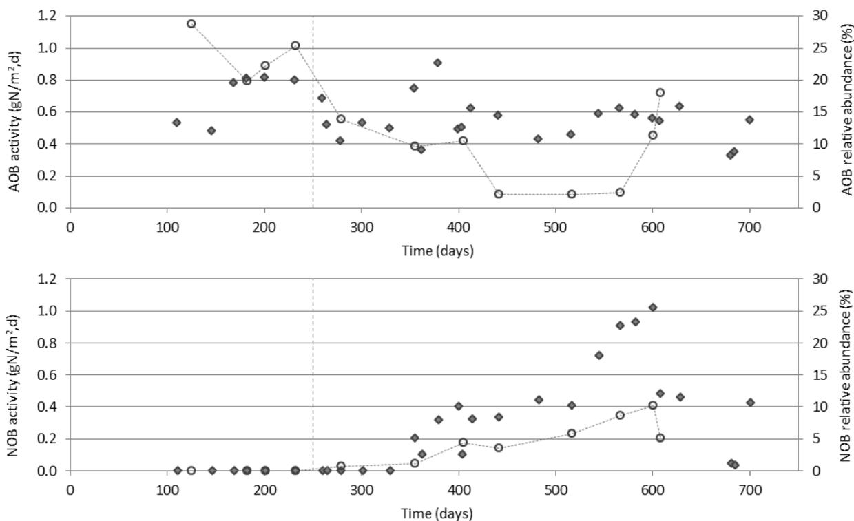
**Figure 13: Observed activity in batch trials (diamonds) and relative abundance from DNA sequencing (circles) of AOB (top) and NOB (bottom) in carriers from the N-stage over time. Dashed vertical line represents switch to mainstream operation.**
