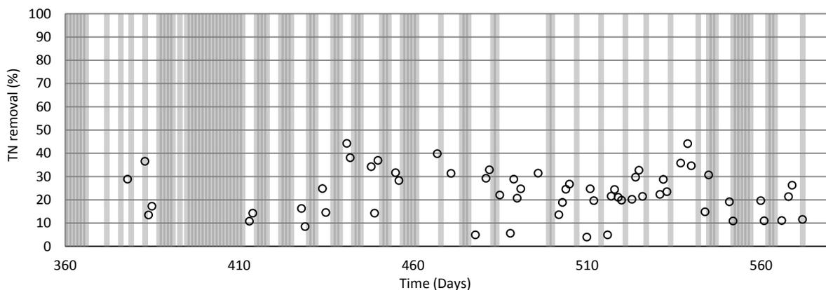
**Figure 12: Total nitrogen removal (%) in the two-stage process during mainstream operation (vertical grey lines represent days with reject operation when anammox stage was bypassed except during day 390-410 were the AMX-stage was fed reject water)**
