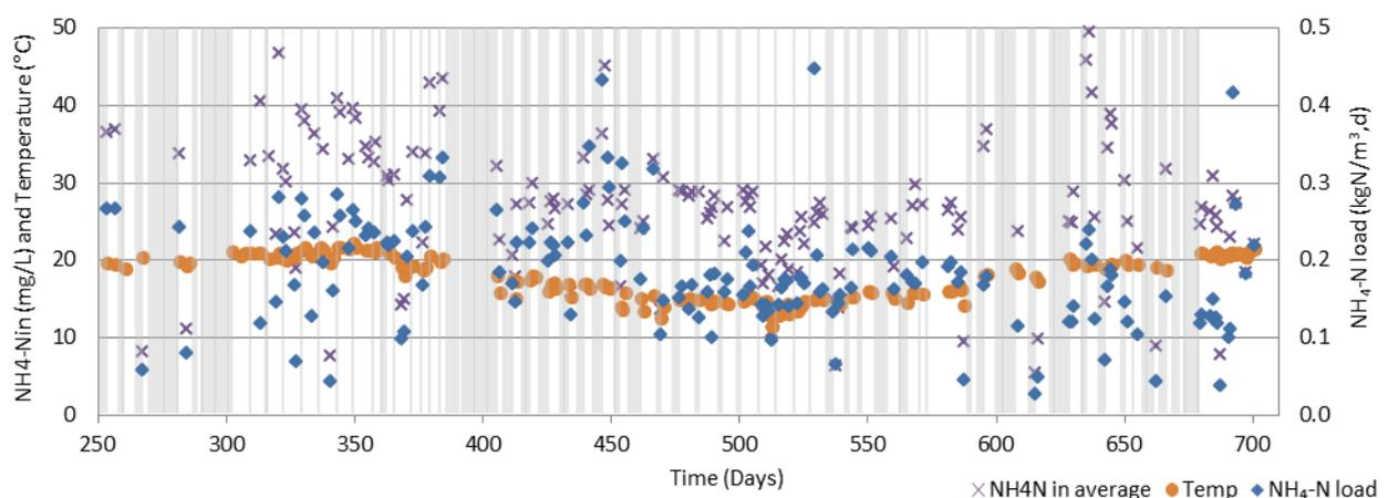
**Figure 7: Characteristics of the inlet water to the N-stage over time during mainstream operation (vertical grey lines represent days with reject feed).**
