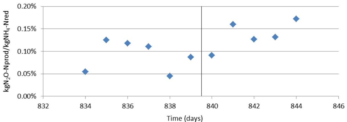
**Figure 23: Produced N<sub>2</sub>O-N over reduced NH<sub>4</sub>-N over time. The black line represents the time when the feed was changed to effluent from the Hydrotech drumfilter.**
