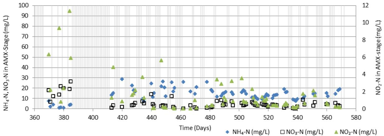
**Figure 11: Reactor concentrations in the AMX-stage during continuous operation on mainstream water (vertical grey lines represent days with reject operation when the AMX-stage was by-passed except during day 390-410 were the AMX-stage was fed reject water)**
