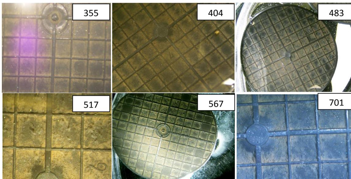
**Figure 16:** The biofilm on Anox K™ Z-200 carriers from the N-stage seen from above using a stereomicroscope on different operational days during mainstream operation.
