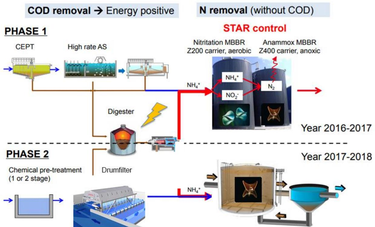
Figure 4: The two phases for the N removal using the HRAS effluent and two-stage nitritation + anammox configuration in phase 1 and Hydrotech Drumfilter effluent and one-stage IFAS configuration in phase 2.
