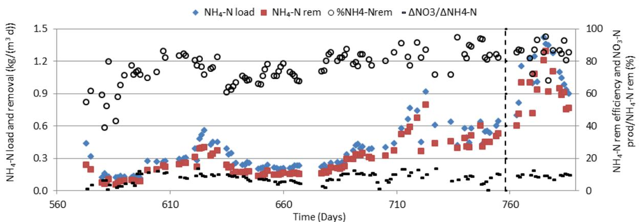
**Figure 18: Ammonia load, ammonia removal and produced nitrate over reduced ammonia during reject water feed. The dashed line on day 758 represents the day when the settler was connected to the MBBR.**
