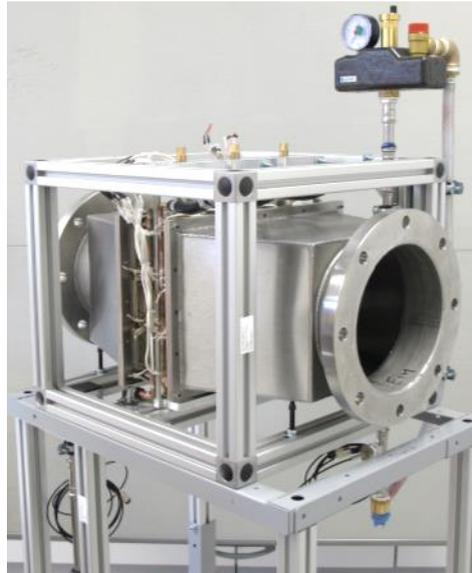
**Figure 16: Thermoelectric generator prototype for Braunschweig case study**
