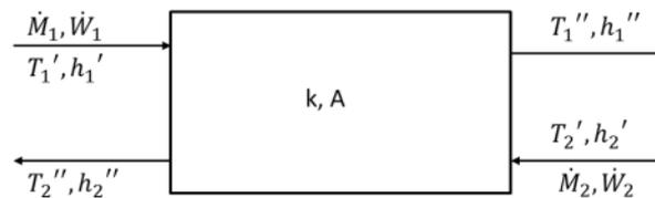
Figure 10: Schematic diagram of a heat exchanger [18]
