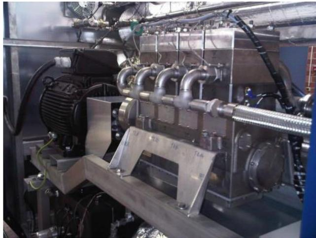
**Figure 5: HT SRC unit with 4-cylinder piston expander.**
