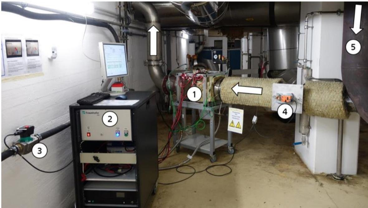
**Figure 27: Overview of the TEG with electronic control unit/measurement electronics.** 1: TEG; 2: electronic rack with MPPTs, electronic load, data acquisition unit; 3: coolant pump; 4: rapid-action exhaust gas valve; 5: main exhaust pipe of standard heat exchanger by-pass; arrows indicate the flow direction of the exhaust gas (photo taken 07.11.17).
