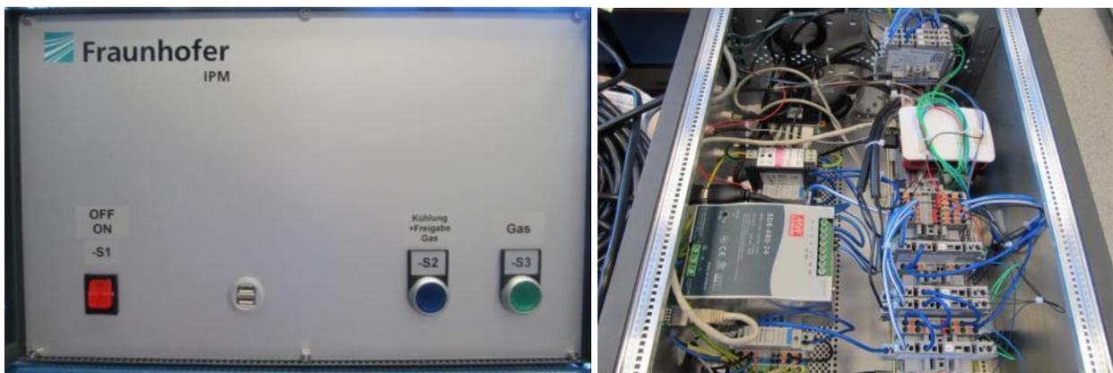
Figure 21: Measurement system with Raspberry Pi B3 single board computer. Left: Front panel, Right: Internal wiring
